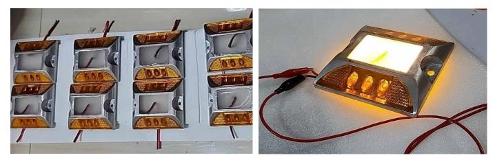
(Above left 04 and right 05) For the flashing devices, the study uses King Kong aluminum stud lights as a shell, but since they usually do not have a flashing element installed, the study commissioned an additional LED flash unit that was custom designed and built that can fit into the shell neatly, and lastly a clear resin coat was used to encase and protect the overall unit.
