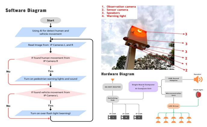
(Above left 09) Software diagram illustrating the operational sequence of the software system, how it detects movement and its activation of the flash lights and sirens. (top right 10) close-up image of the electronic housing which contains the hardware within, and on the exterior, it acts as the main mount for the sensors, cameras and speakers for the sirens. (bottom right 11) Hardware diagram showing how the systems are interconnected with the software.
