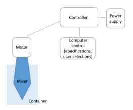
This prototype enabled the testing of parameters associated with different liquid thickness categories (thin, slightly thick, mildly thick, moderately thick, extremely thick) specified by the International Dysphagia Diet Standardization Initiative (IDDSI). This would allow objective and automatic categorization of liquid thickness for the end-user.
