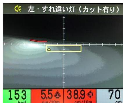
Fig.5 In the low beam after switching, the elbow point of the left and right of the light has been irradiated in the upper left direction, it does not meet the compliance range.
