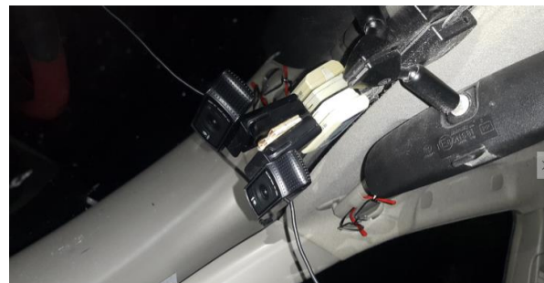
Fig. 5: Camera unit attached on windshield
