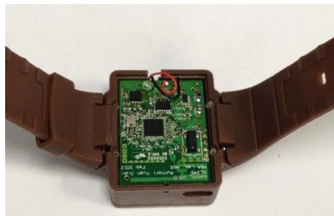
Figure 5: Wearable Device Embedded into a Watch Case
