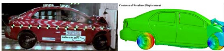
Figure 1 shows a comparison of the global deformation behaviour of the crashed car
