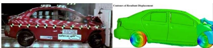
Figure 1 shows a comparison of the global deformation behaviour of the crashed car
